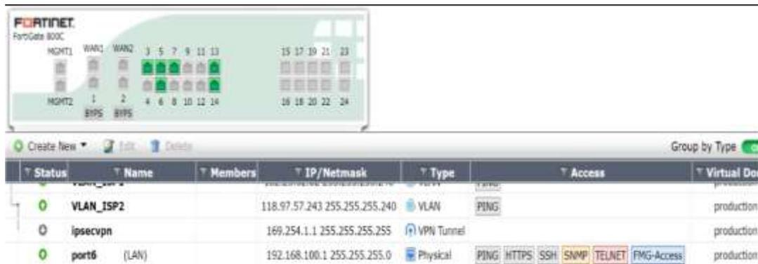
**Figure. 5** Configuration of Fortigate for the management port
