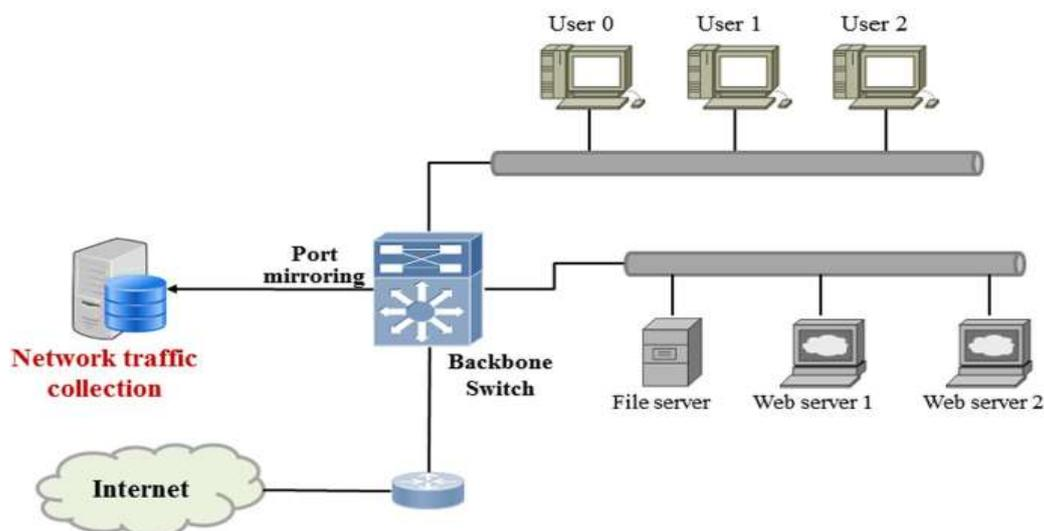
Figure. 2 Schematic diagram of network traffic in real time.
