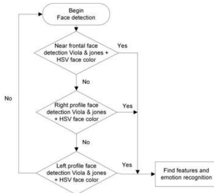
**Figure. 4** Flowchart for multi view face detection
